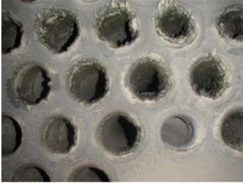
The tubes are in a really bad condition. The deposits are solid, bonded to the metal and very difficult to remove. Abrasive de-scaling had to be used to clean the tube. Their must be considerable fuel losses.
