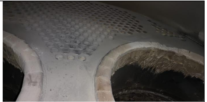
Whitish appearance of tubes due to catalytic effect of Sapec.
